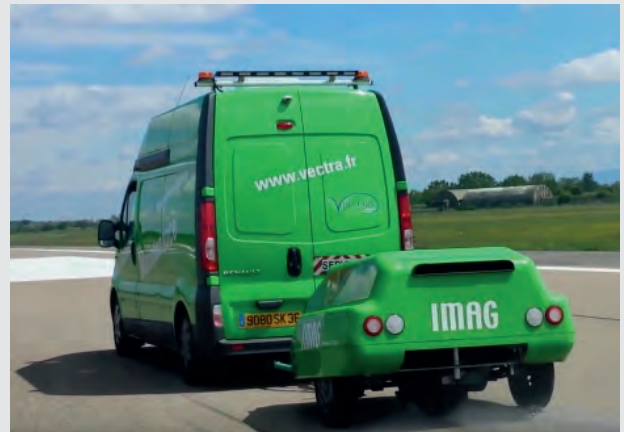
Video of Vectra IMAG carrying out LFC measures.
